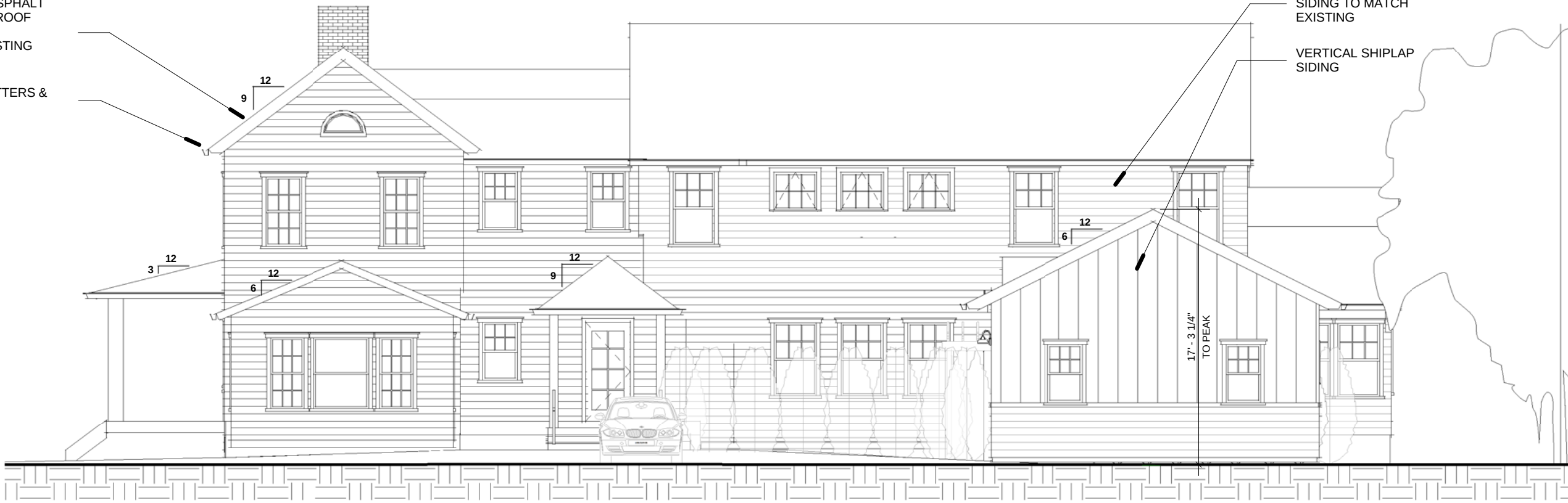
PROPOSED EAST ELEVATION 3/16" = 1'-0"
