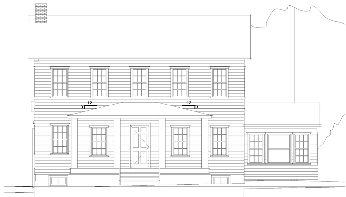
EXISTING SOUTH ELEVATION 3/16" = 1'-0"
