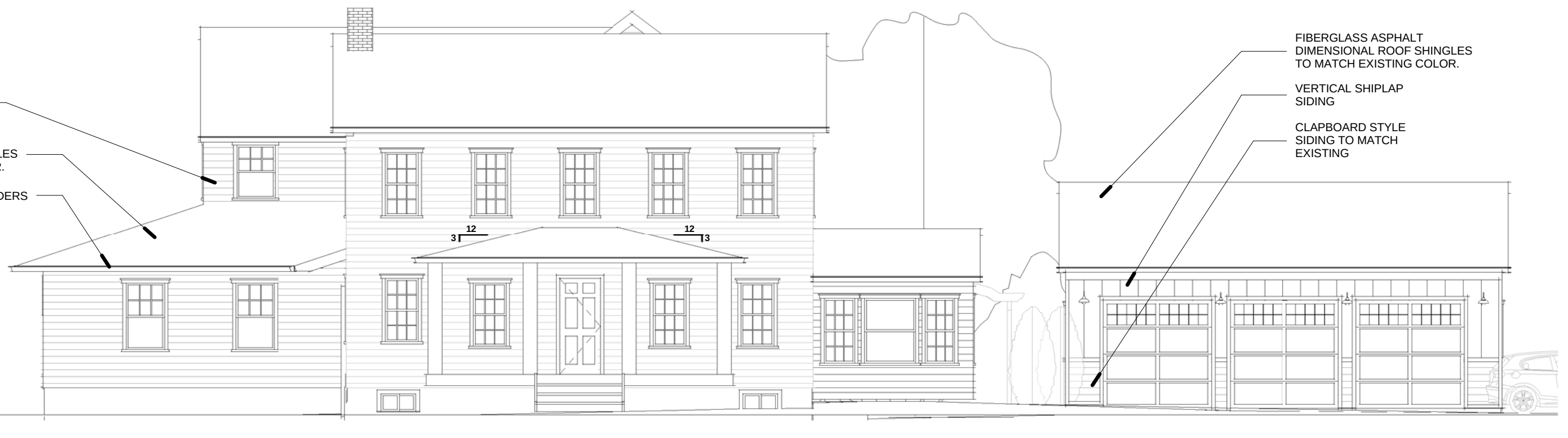
PROPOSED SOUTH ELEVATION 3/16" = 1'-0"
