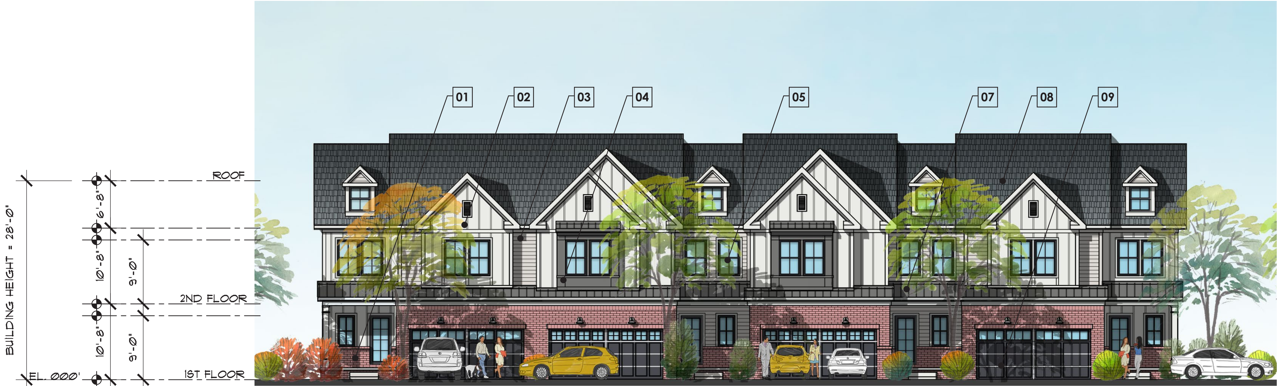
01 - 30' MASTER DOWN TH FRONT LOADED - TYPICAL FRONT ELEVATION SCALE: 1/8" = 1'-0" 0 4' 8' 16'
