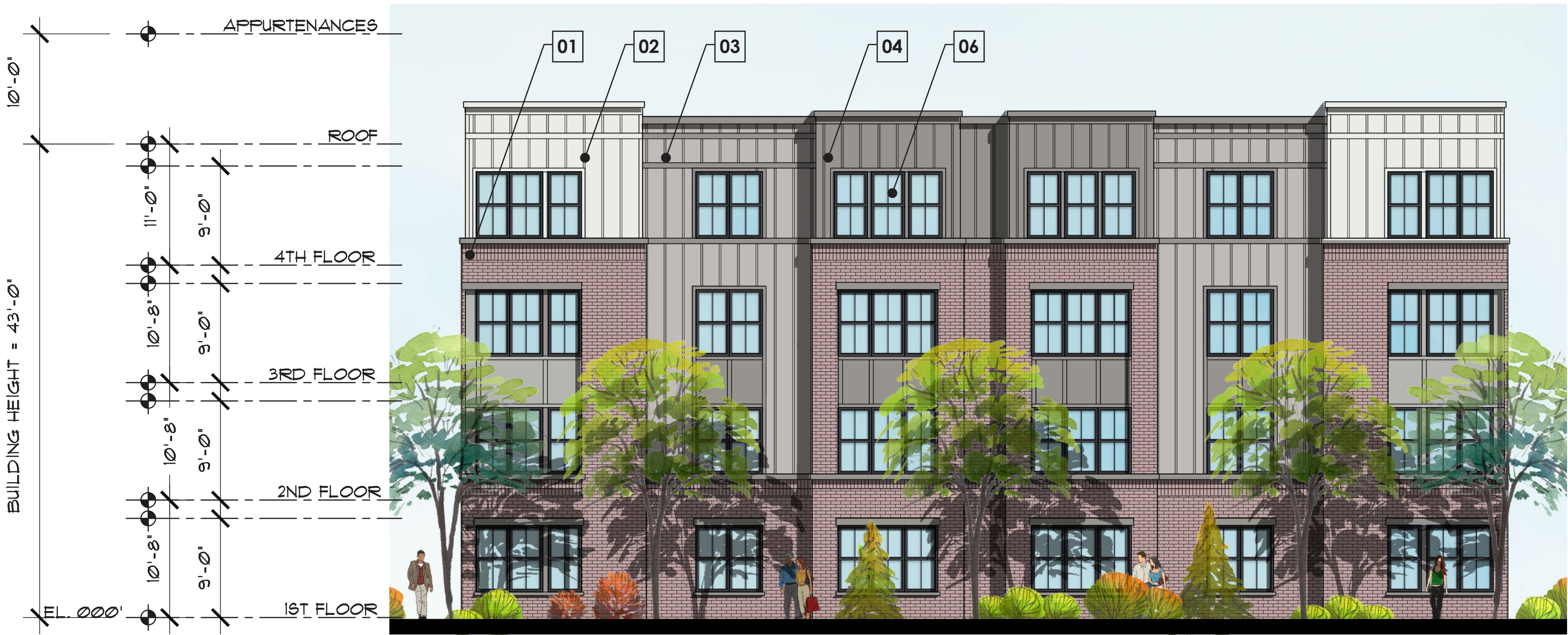
02 - MULTIFAMILY FLATS - TYPICAL LEFT SIDE ELEVATION SCALE: 1/8" = 1'-0" 0 4' 8' 16'
