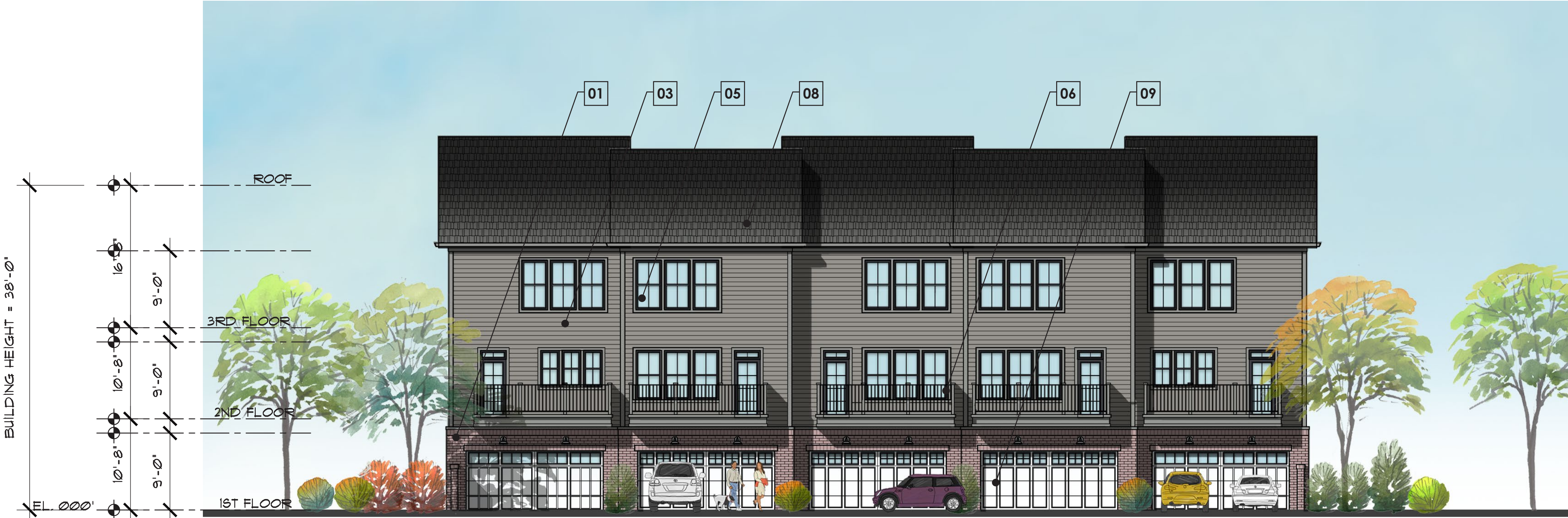
01 - 20' TRADITIONAL TH REAR LOADED - TYPICAL REAR ELEVATION
