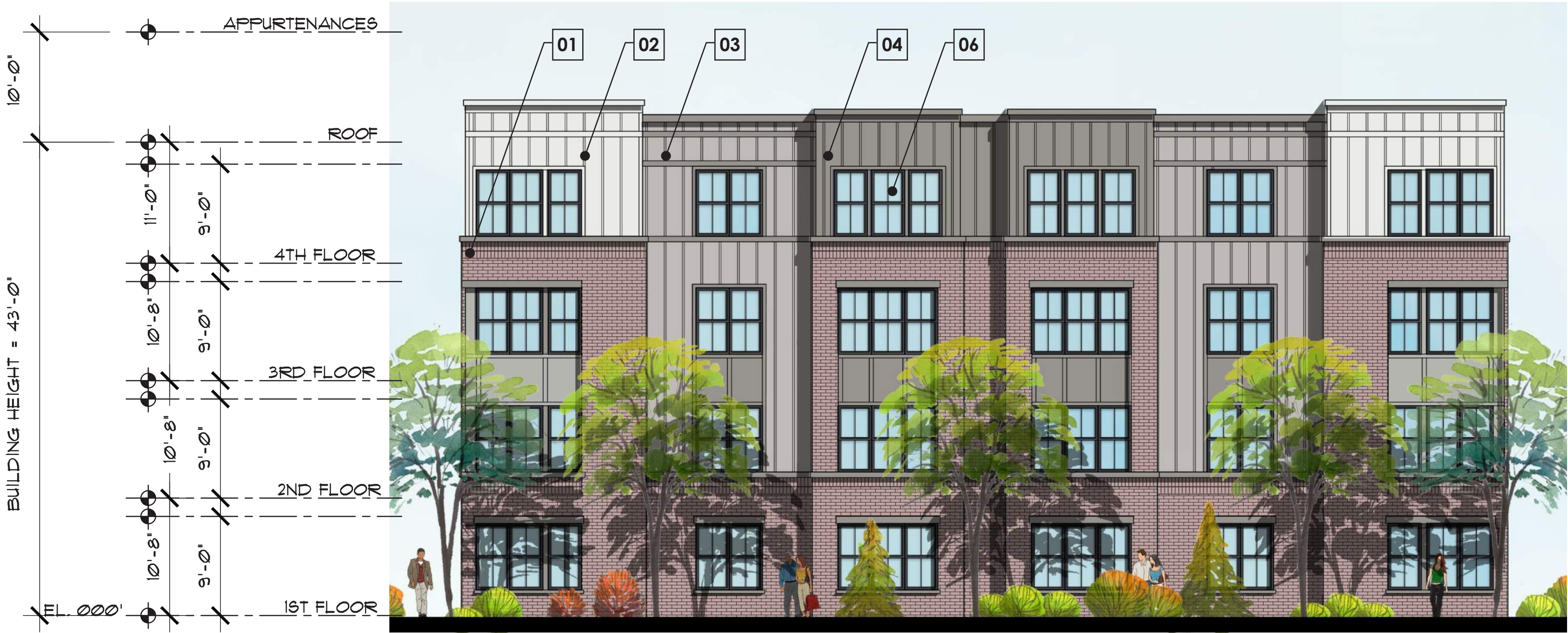
02 - MULTIFAMILY FLATS - TYPICAL LEFT SIDE ELEVATION SCALE: 1/8" = 1'-0" 0 4' 8' 16'
