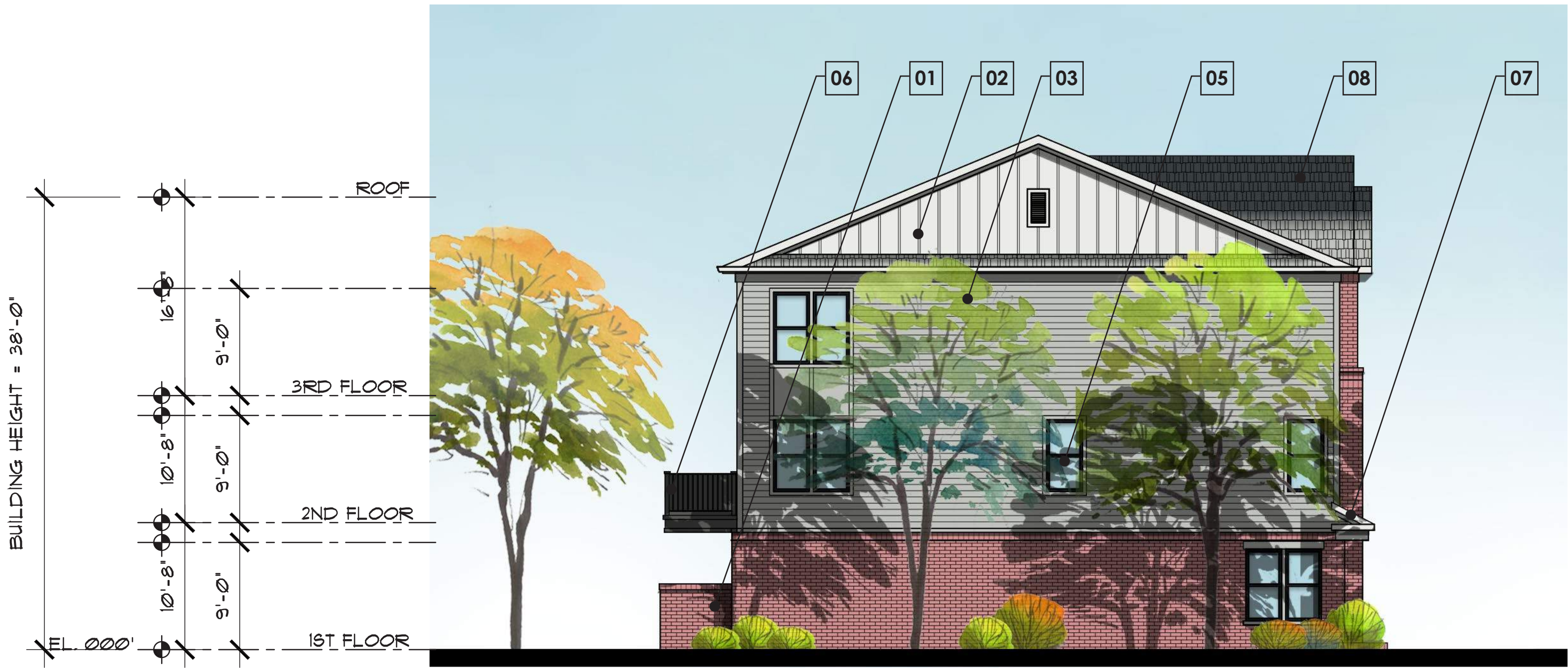
02 - STACKED TOWNHOMES - TYPICAL LEFT SIDE ELEVATION SCALE: 1/8" = 1'-0" 0 4' 8' 16'
