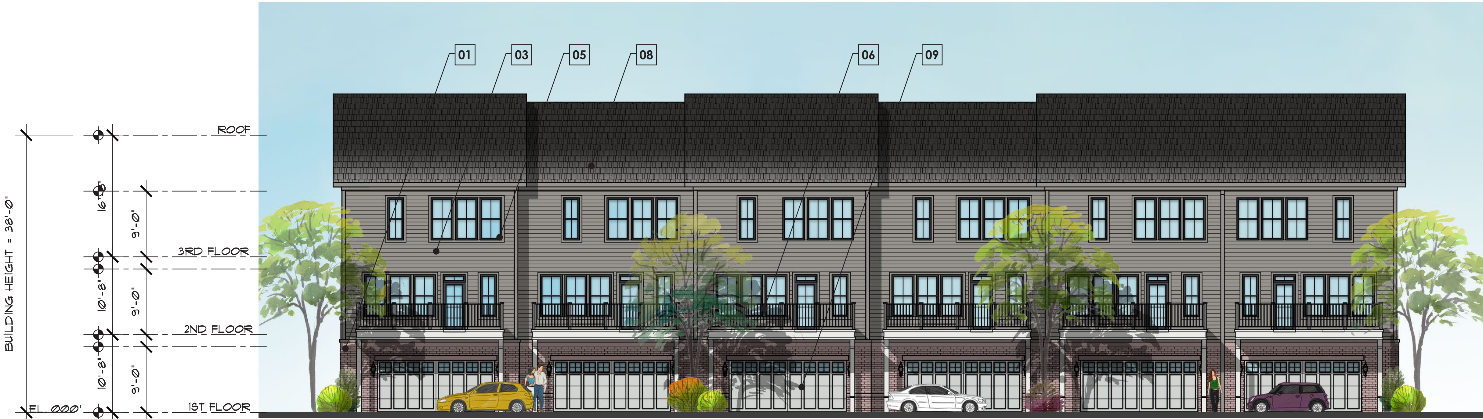
01 - 24' TRADITIONAL TH REAR LOADED - TYPICAL REAR ELEVATION SCALE: 1/8" = 1'-0" 0 4' 8' 16'
