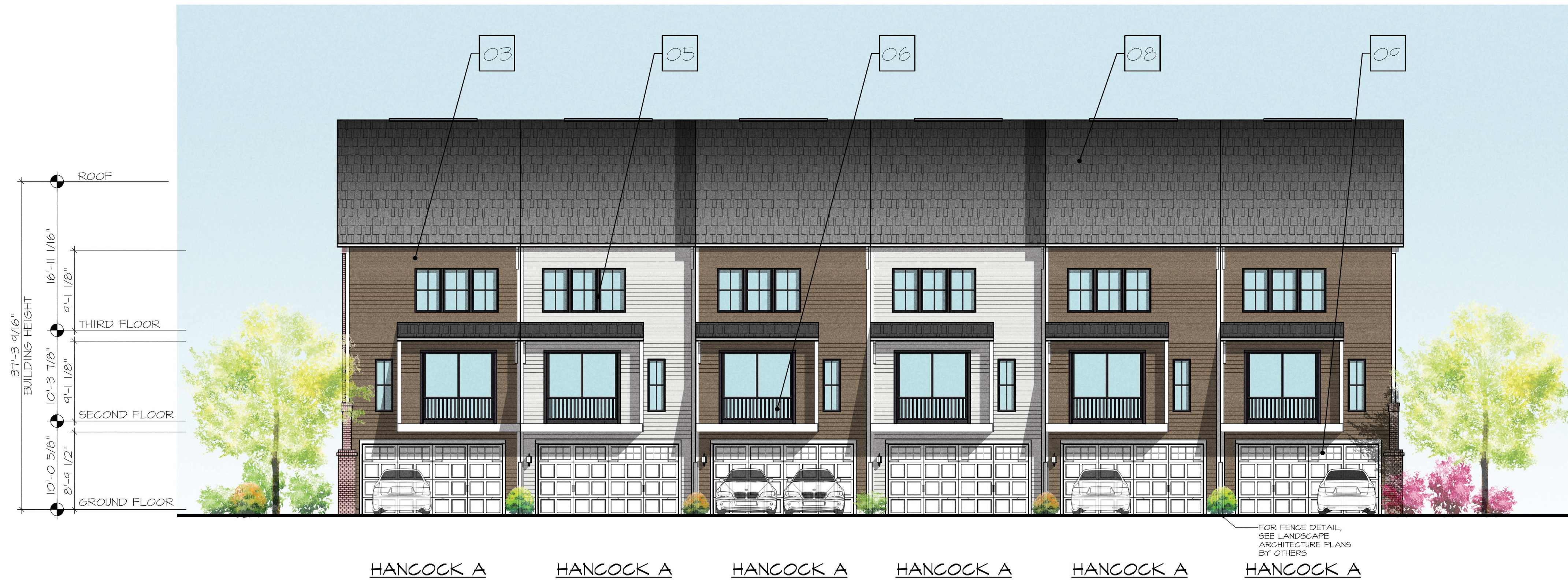
1 A-3 6-UNIT BUILDING REAR ELEVATION SCALE: 1/8" = 1'-0"
